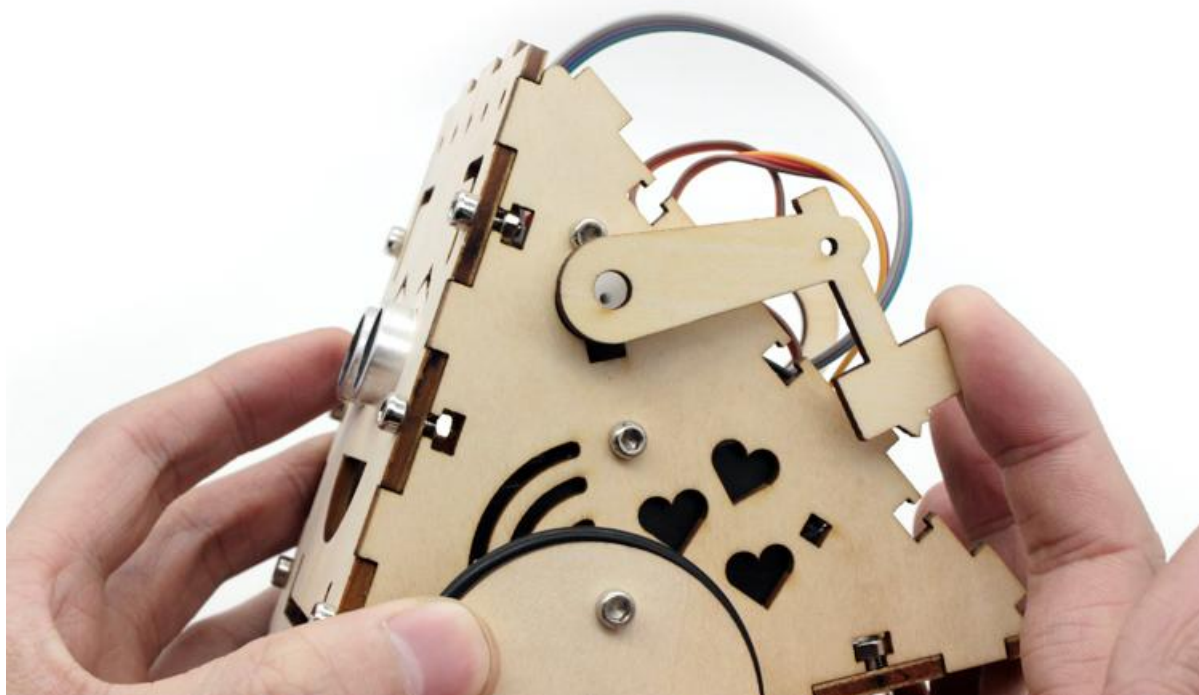
STEP50:Installing the robot arm on the right side, arm in the limit position, pay attention to the position, in the middle;
