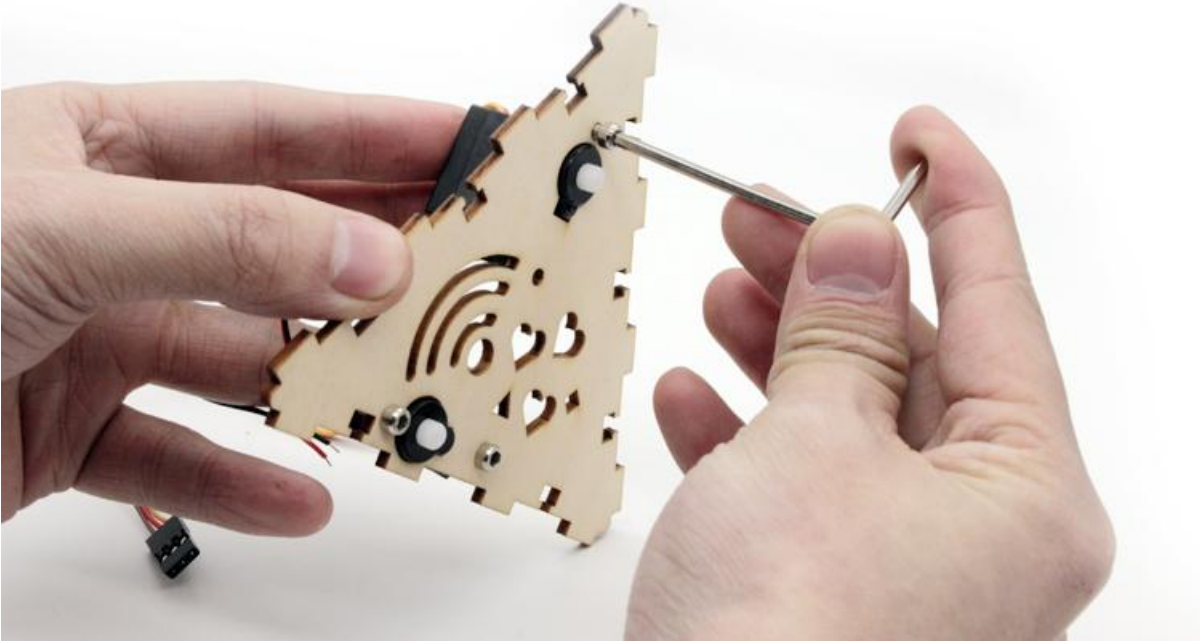
STEP7:Install M3X12 socket head cap screw to the steering arm, pay attention to the first preloaded, after fastening!
