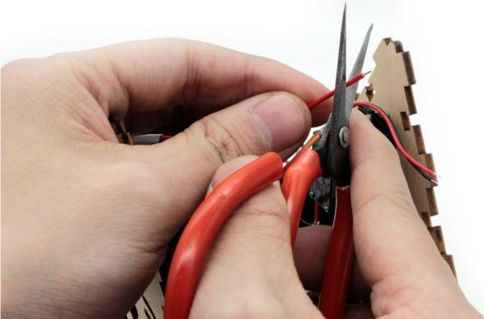
STEP19:With scissors to remove battery pack wire insulation
