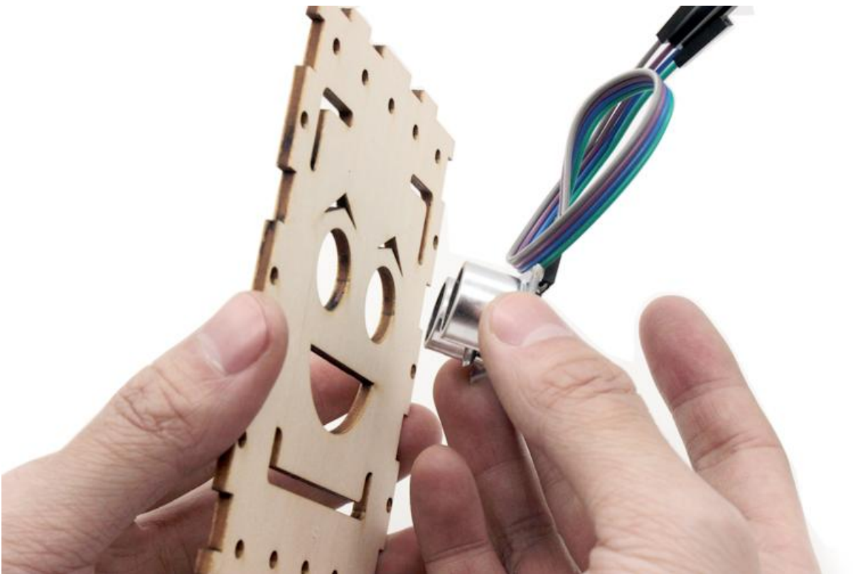
STEP24:Install the eye to the hole of the board, as shown.
