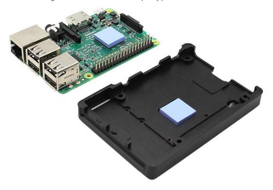
7. Put the Raspberry Pi into the case, remove the protective film of the dark acrylic plate, and put it to the side of the case,install the lower cap.
