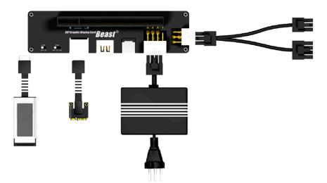
The other end is connected to the data line interface board corresponding to the "reference chart". The HDMI EXP GDC board can not be connected with other HDMI data line, otherwise it will cause equipment damage.
