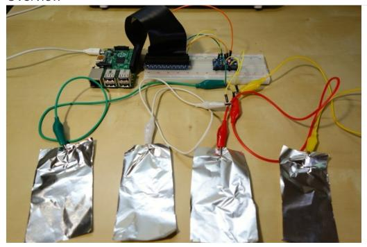
Reach out and touch someone, or some*thing*, with the MPR121 capacitive touch sensor and a Raspberry Pi or BeagleBone Black! This breakout provides 12 capacitive touch inputs and all the logic to read them over a simple I2C communication bus. For example you can make your own buttons, detect if someone touched a device, create a fun plush game controller (https://adafru.it/ne8), or even a wacky devices like a banana piano (https://adafru.it/eid)!
